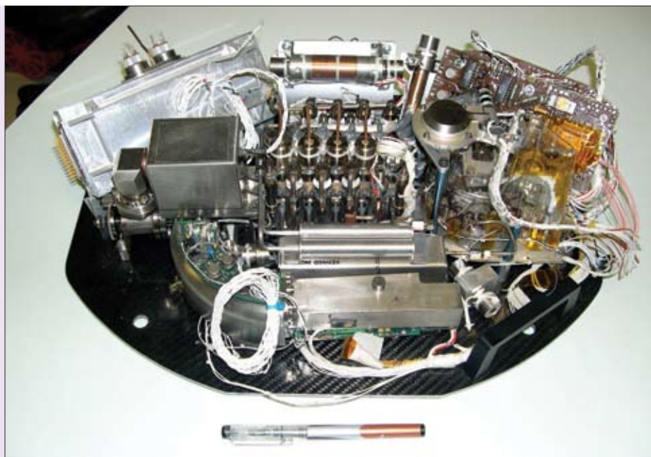
2: The Gas Analysis Package (GAP) developed for the Beagle2 mission. Such an instrument, incorporated into future lunar missions, would be ideal for detecting and characterizing volatile and organic substances in the lunar regolith. (Everett Gibson/OU/Beagle2)
